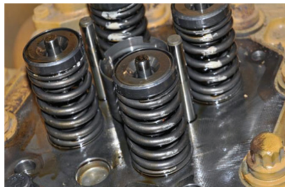
Caterpillar G3516 TALE E+ valve springs at end of Approval Test (8,089 hours)
